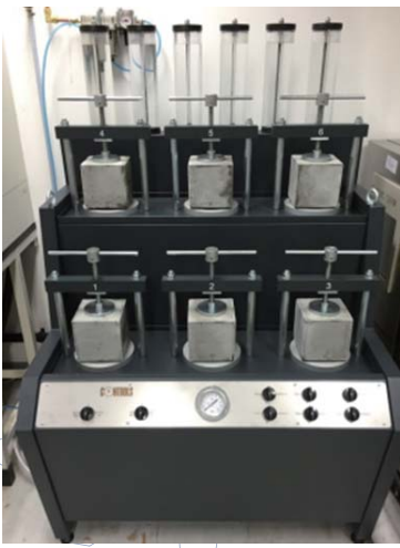
Water permeability apparatus
