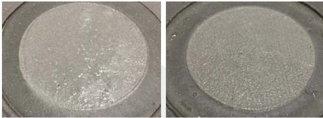
It is easy to find the coating blistering when the coatings are exposed to the water with pressure of 5 Bar over 72 hours.
