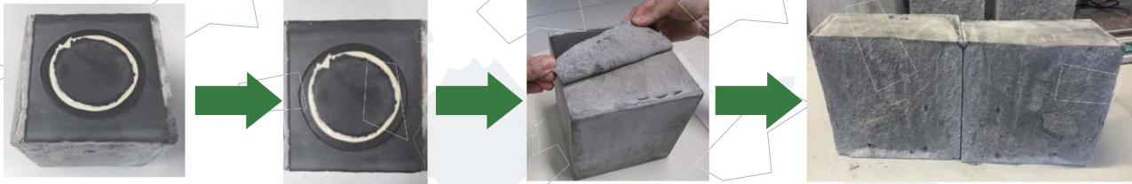
Investigation of depth of water penetration under 5 Bar water pressure for 72 hours. No water penetration was found.
